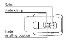
Loosen the blade se cur ing bolt fully with the hex wrench. Keep the back edge of the blade fit ting into the roller and in sert the blade be tween the blade clamp and the slider as far as it will go.l Make sure that you are in sert ing the blade into the proper posi tion.
